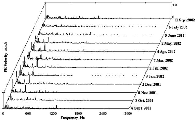
Fig. 16. Multiple spectrum graph of the fan motor outer bearing.
