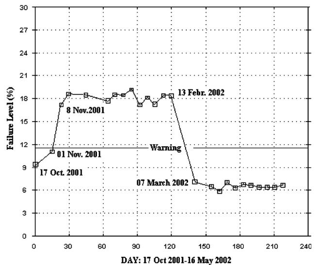
Fig. 7. Overall vibration level trend of the pump inner bearing.
