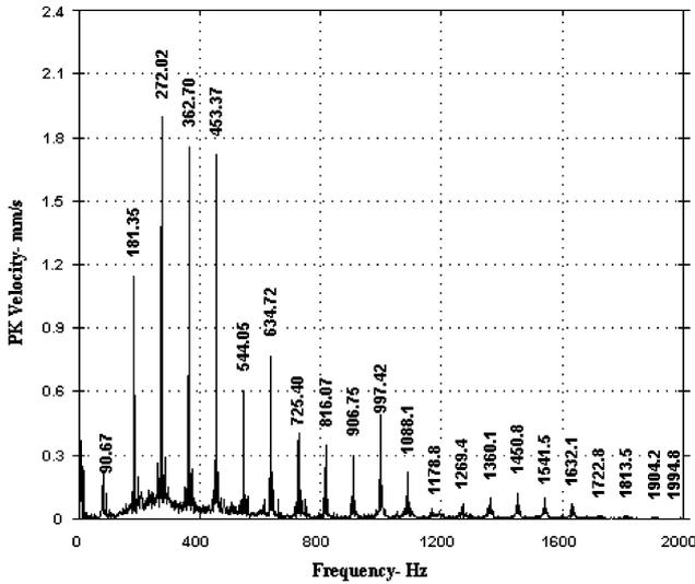
Fig. 9. Reference spectrum graph of the fan motor inner bearing.
