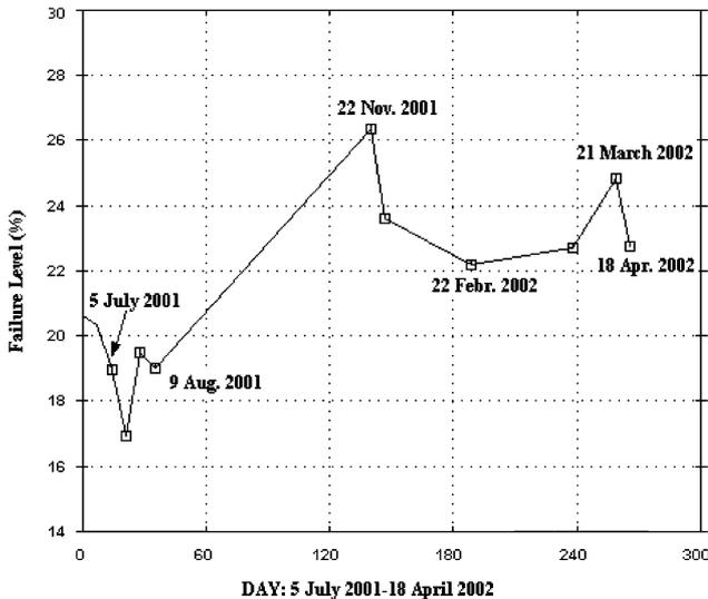
Fig. 10. Overall vibration level trend of the fan motor inner bearing.
