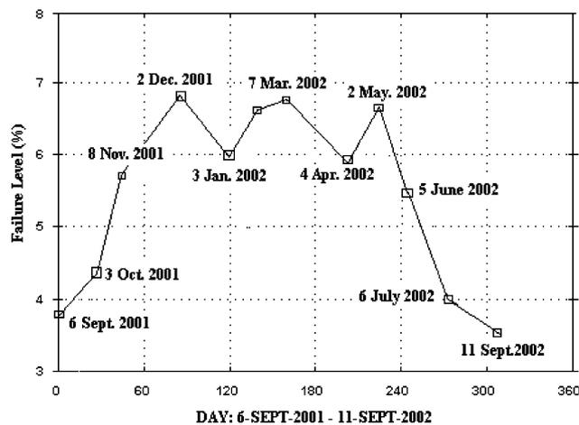
Fig. 17. Overall vibration level trend of the fan motor outer bearing.
