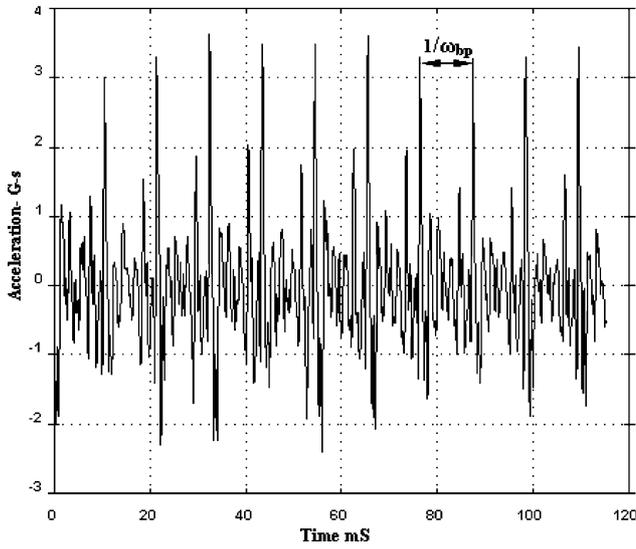
Fig. 8. Reference time domain waveform graph of the fan motor inner bearing.
