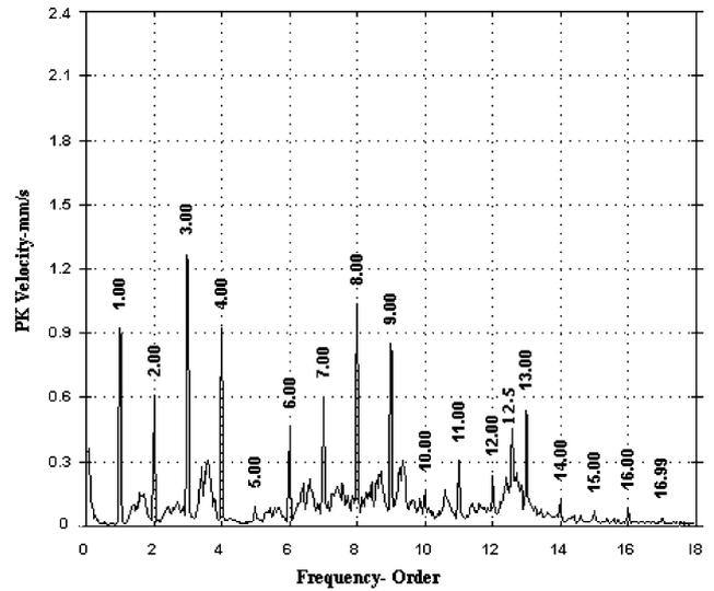
Fig. 5. Vibration time waveform graph resulted from increasing of looseness.
