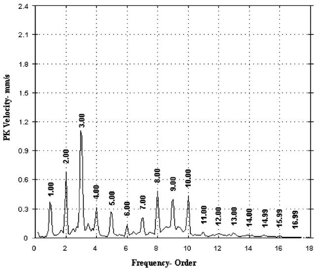
Fig. 3. Reference spectrum graph of the pump inner bearing.
