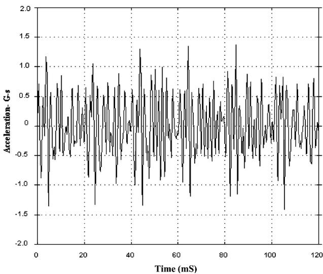
Fig. 4. Vibration time waveform graph resulting from increasing of looseness.
