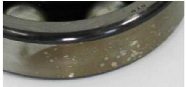
Fig. 6. Corrosion on the ball bearing outer race due to looseness.
