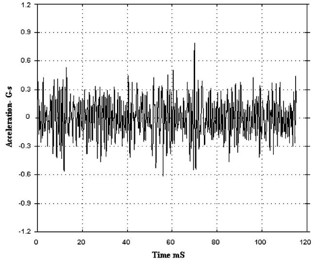
Fig. 11. Reference time waveform graph of the fan motor outer bearing.
