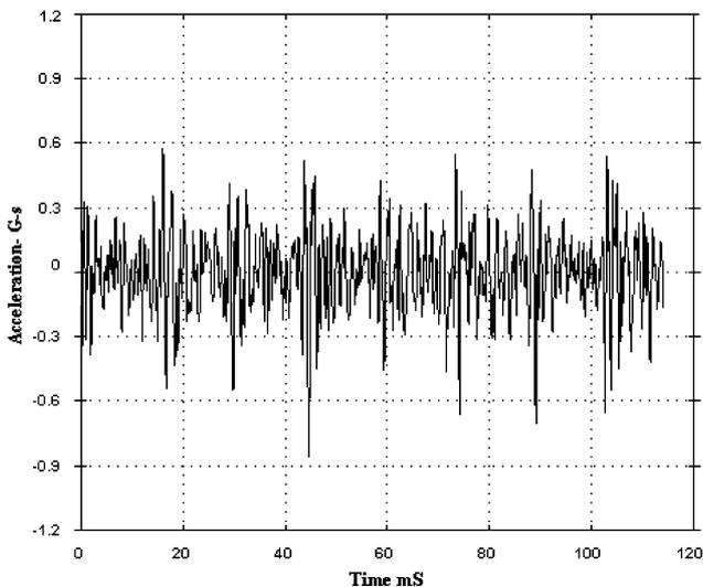
Fig. 13. Time waveform graph of the fan motor outer bearing on 3 October 2001.
