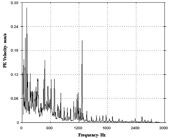
Fig. 12. Reference spectrum graph of the fan motor outer bearing.
