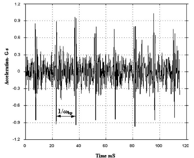
Fig. 15. Time waveform graph of the fan motor outer bearing on 6 July 2002.
