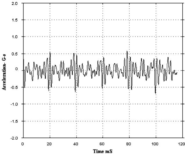
Fig. 2. Reference time waveform graph of the pump inner bearing.
