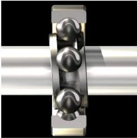
Figure1: Inner race cocked on the shaft
