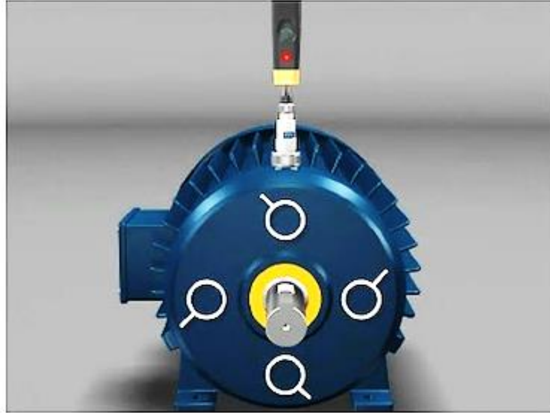
Figure3: Phase changes when the bearing is cocked on the shaft
