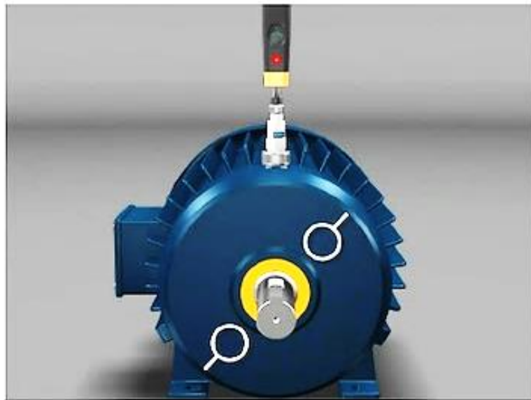
Figure4: Phase changes when the bearing is cocked in the housing
